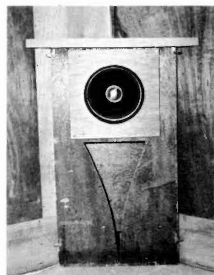
Fig. 9. Semi-finished cabinet with loudspeaker in place on its mounting panel. Note brackets on edges of front panel for mounting the trimming frame.
