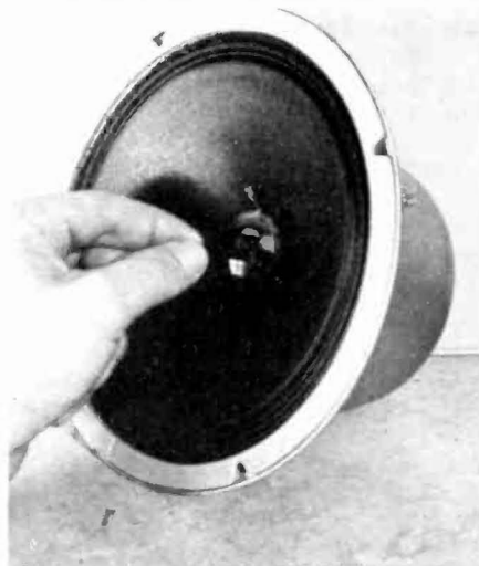
Fig. 3. Inserting shims to hold the voice coil in position.
