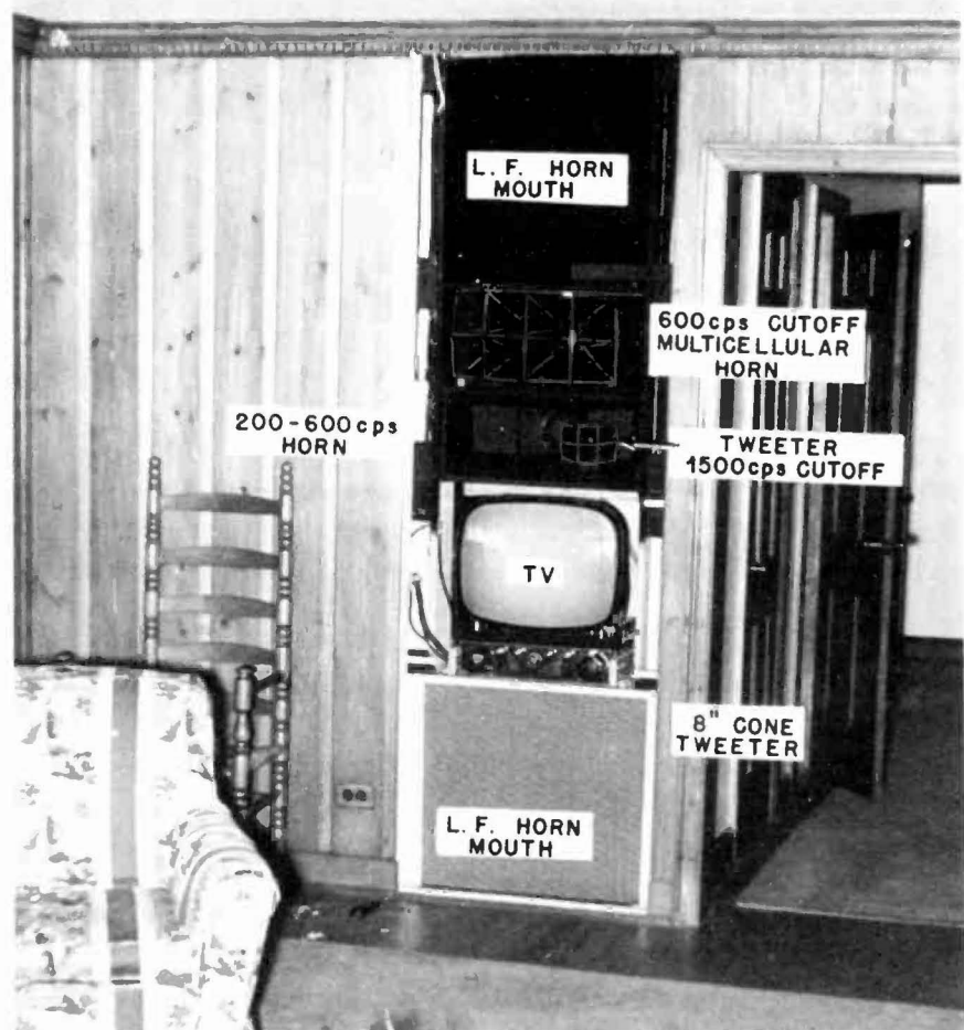
Fig. 1. The finished enclosure is mounted in a closet with the divided horn exhausting into the listening area. Between the two sections is the TV receiver. The upper section will be covered with a grill similar to that over the lower section.
