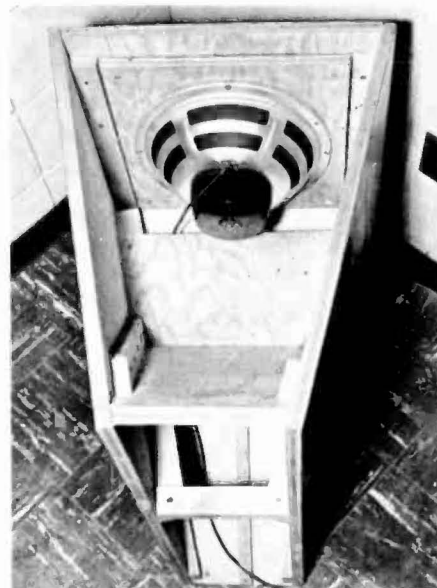
Fig. 3. This view of the enclosure turned around from its normal position, was taken from above and behind. It is useful in showing many details, though somewhat deceptive from a photographic standpoint. To avoid misunderstanding, remember that the side walls are rectangular, the top parallel to the floor.
