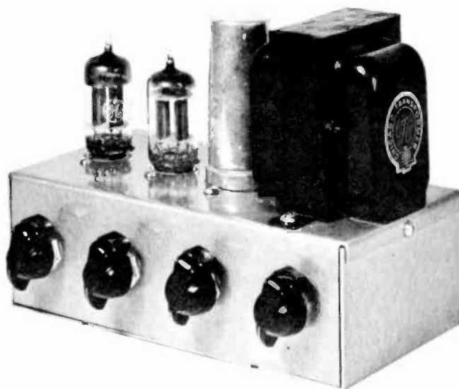
Fig. 4. Three-element bass-boost circuit with self-contained power supply.
