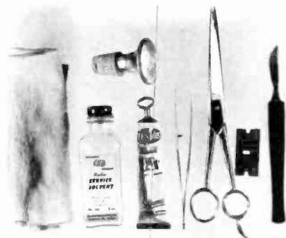
Fig. 1. Materials needed for treating speakers—chamois, solvent, cement, tweezers, scissors, razor blade, scalpel, and in some cases clothes-sprinkler head.
